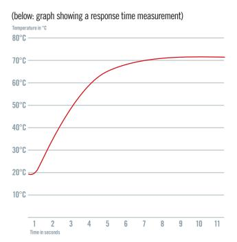
Depending on the type of hot junction used, the characteristic response times which can be obtained are indicated below:
