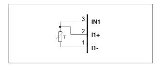
Figure 20 Connection diagram for 1V/20mA linear input
