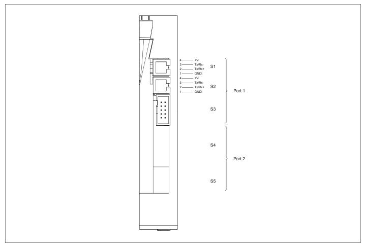
Connector S3 to connection to STATOP 704 slave modules
