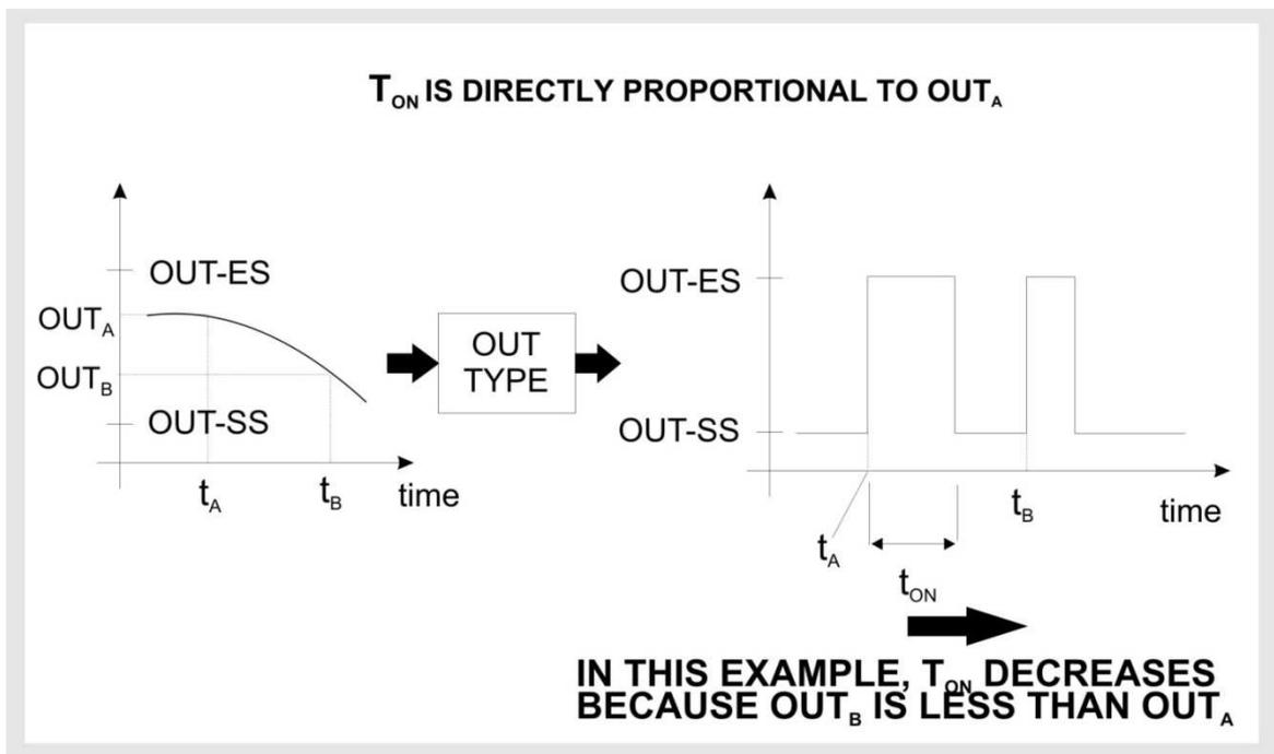
It is possible to limit inferiorly the time of high-state ON/OFF output (reg.40029) and to limit inferiorly the time of low-state ON/OFF output (reg.40030). The cycle time is reg.40028 (constant frequency of ON/OFF output=1/cycle time).
