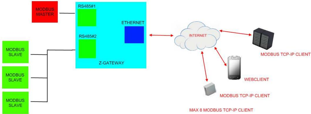
**Shared Memory: RS485#1 and RS485#2 Modbus RTU Slave, Ethernet Modbus TCP-IP server (200 Modbus Registers that can be written and read from a Modbus RTU Master or Ethernet Modbus TCP-IP server, for example:**
