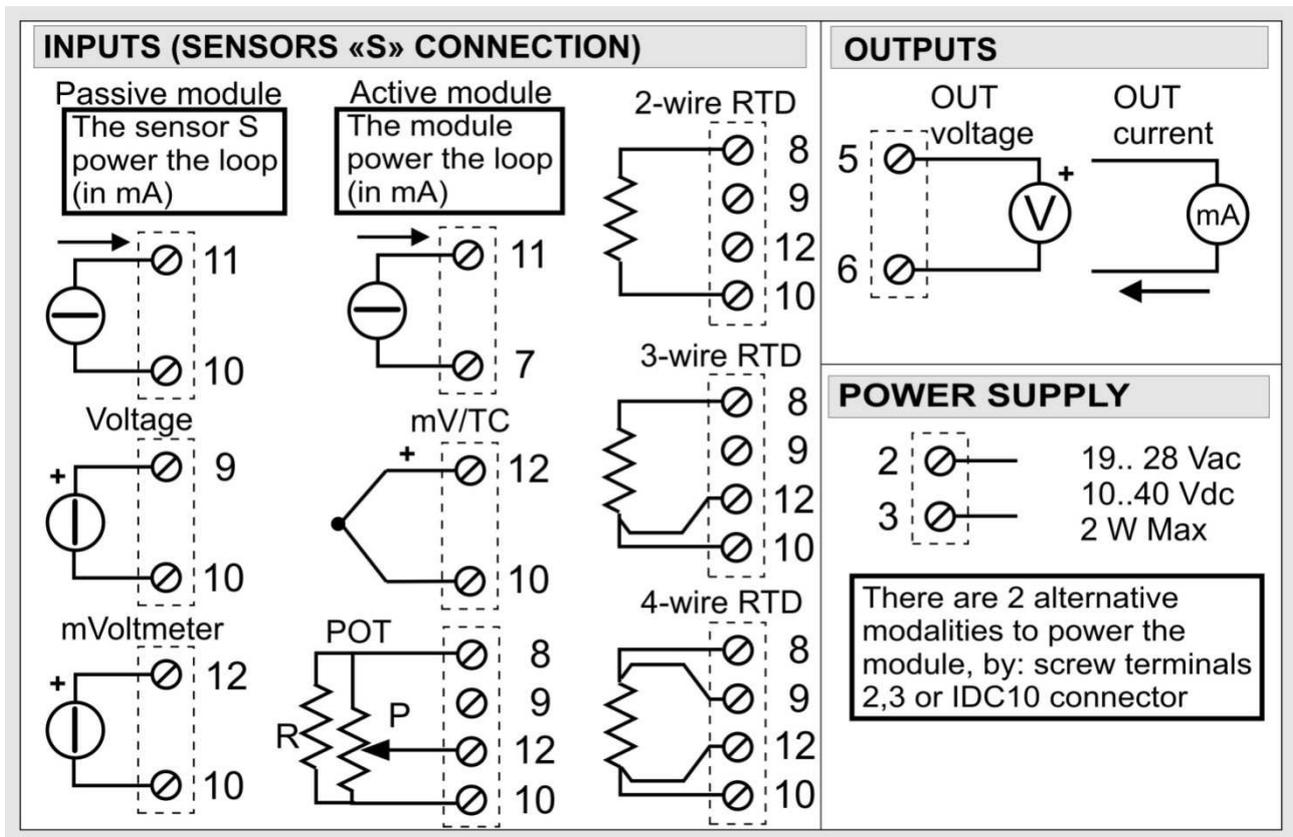
For potentiometer input connection: with  $R=330 \Omega$  ( $R$  needs to be added externally),  $P=1 \text{ k}\Omega\text{-}100 \text{ k}\Omega$
