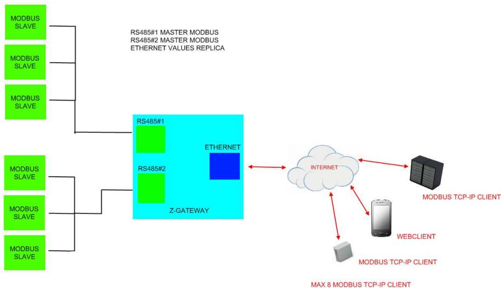
**RS485#1 Modbus RTU Master, replica values on RS485#2 Modbus RTU Slave or Ethernet Modbus TCP-IP server, for example:**
