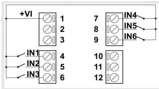
If jumper J1 is in “Ext” position, input screw terminals configuration is shown in the following figure. In this configuration, **a external voltage supply is necessary.**
