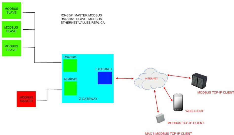
**RS485#2 Modbus RTU Master, replica values on RS485#1 Modbus RTU Slave or Ethernet Modbus TCP-IP server, for example:**
