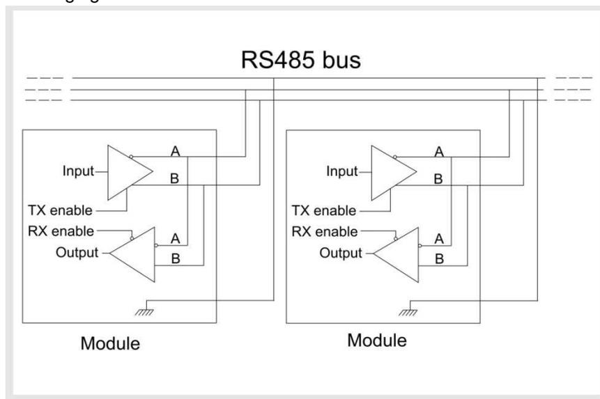
As shown, there are three wires assigned to communication: A, B and GND. This topology allows an half-duplex transmission between electrical-equivalent modules (this means that tx and rx are not enabled at the same time). The PDM modules have an integrated transmitter and an integrated receiver.
