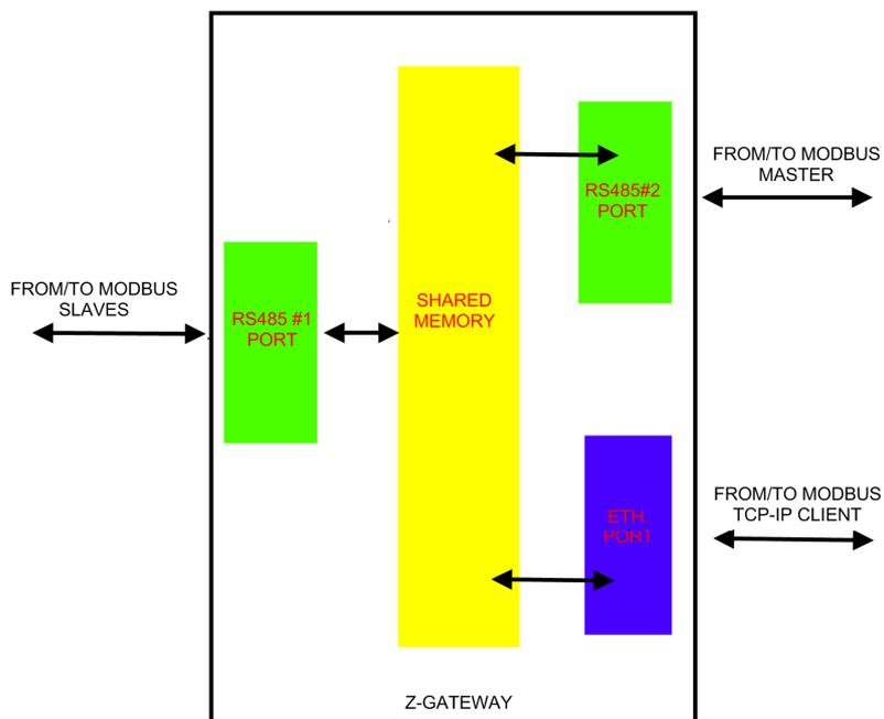
In this way the shared memory is always refreshed at maximum speed from the “slaves side” and the values are read from the “masters side” without waiting a slave response.
